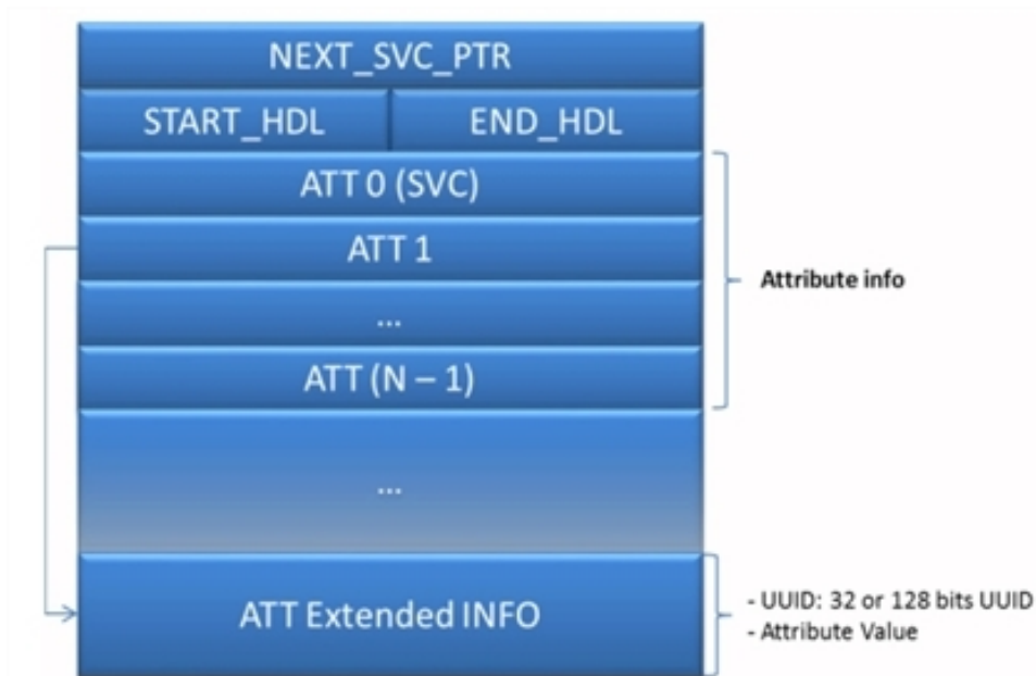
Figure 56. Service Description Block of ATT Database
