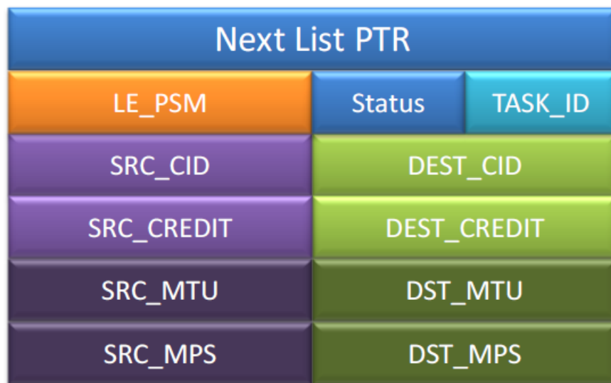
Figure 140. LE Credit Connection Environment Structure
