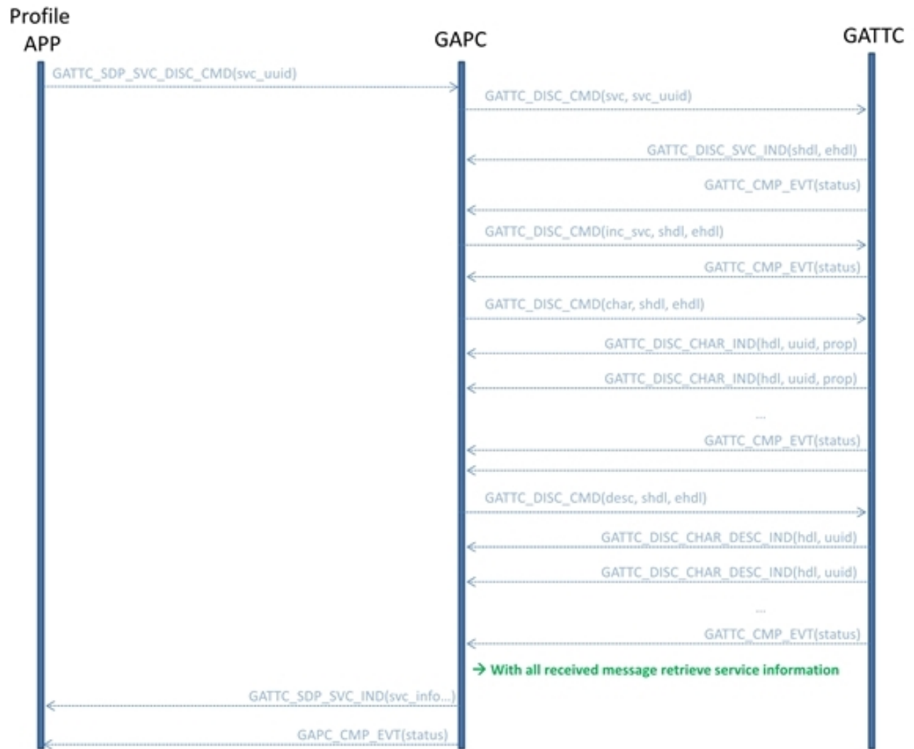
Figure 86. Service Discovery Procedure
